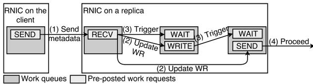
**Figure 7: Datapath of gMEMPCPY primitive.**
