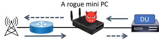
Figure 5: An adversary can intercept and manipulate fronthaul traffic without violating IEEE 802.1X by introducing a rogue server with two network interfaces into the fronthaul network. To stay stealthy, the rogue server can be a mini PC (e.g., GoWin R86S Pro [5]) with low power consumption. It works as a network bridge, enabling the adversary to view and modify the fronthaul traffic. Solid arrows indicate normal traffic, while dashed arrows represent manipulated traffic.
